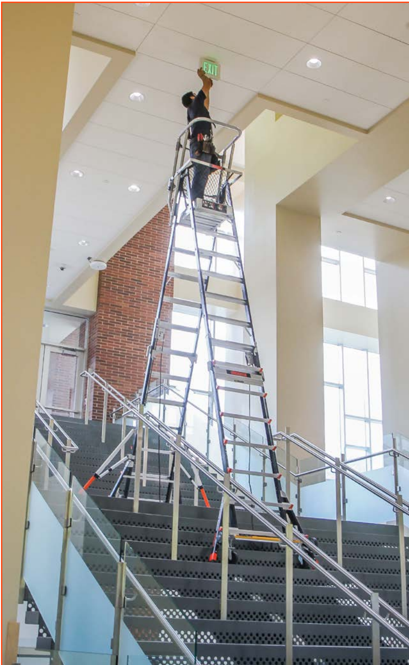
Safe and easy to use on stairs, stadium seating, stages, and other uneven surfaces or at multiple heights.
